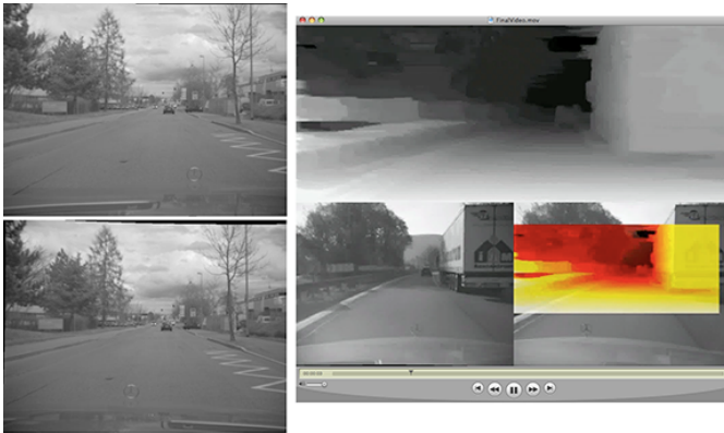
Fig. 6. An illustration for seven stereo night vision sequences available since 2007 on the .enpeda.. website [4] for performance evaluation. Left: one out of close to 2,000 rectified stereo pairs in total. Right: screenshot of an avi showing one original sequence (lower left) and disparity data.
