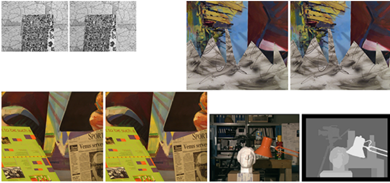
Fig. 5. Illustration of four stereo image sets on the Middlebury vision website: map , sawtooth , venus , and Tsukuba with depth map, illustrating ground truth as available for those data sets on this website
